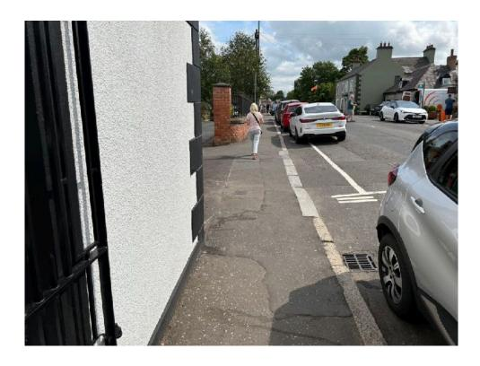
The northern footway narrows to an unacceptable level because of the extended building line of the old bank.
