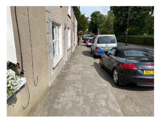
The street has an irregular building line with steps into houses narrowing the footway to unacceptable levels in places.
