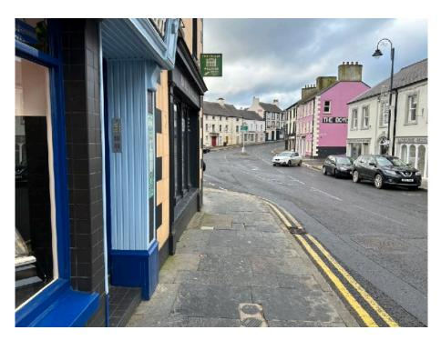
Image shows one of several locations on Ann Street where paving is broken and loose, probably due to pavement parking by heavy goods vehicles.
