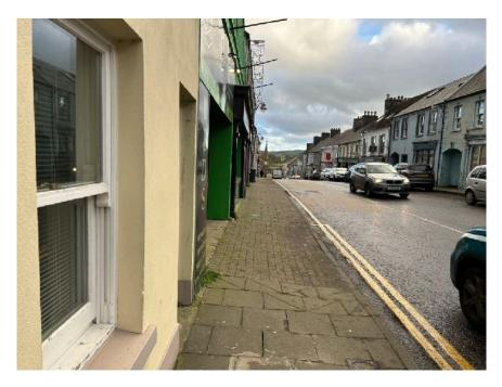
A vehicle entrance on Castle Street creates a sharp drop and crossfall. The surface condition on the footway is also poor in this location.
